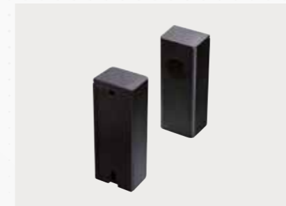
Extra 625 one-way opto sensor 24 V DC, IP 54 Range: 8 m Suitable for: All operator models
